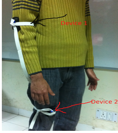
Figure 6: Location of the 2 wireless sensor motes on the body
